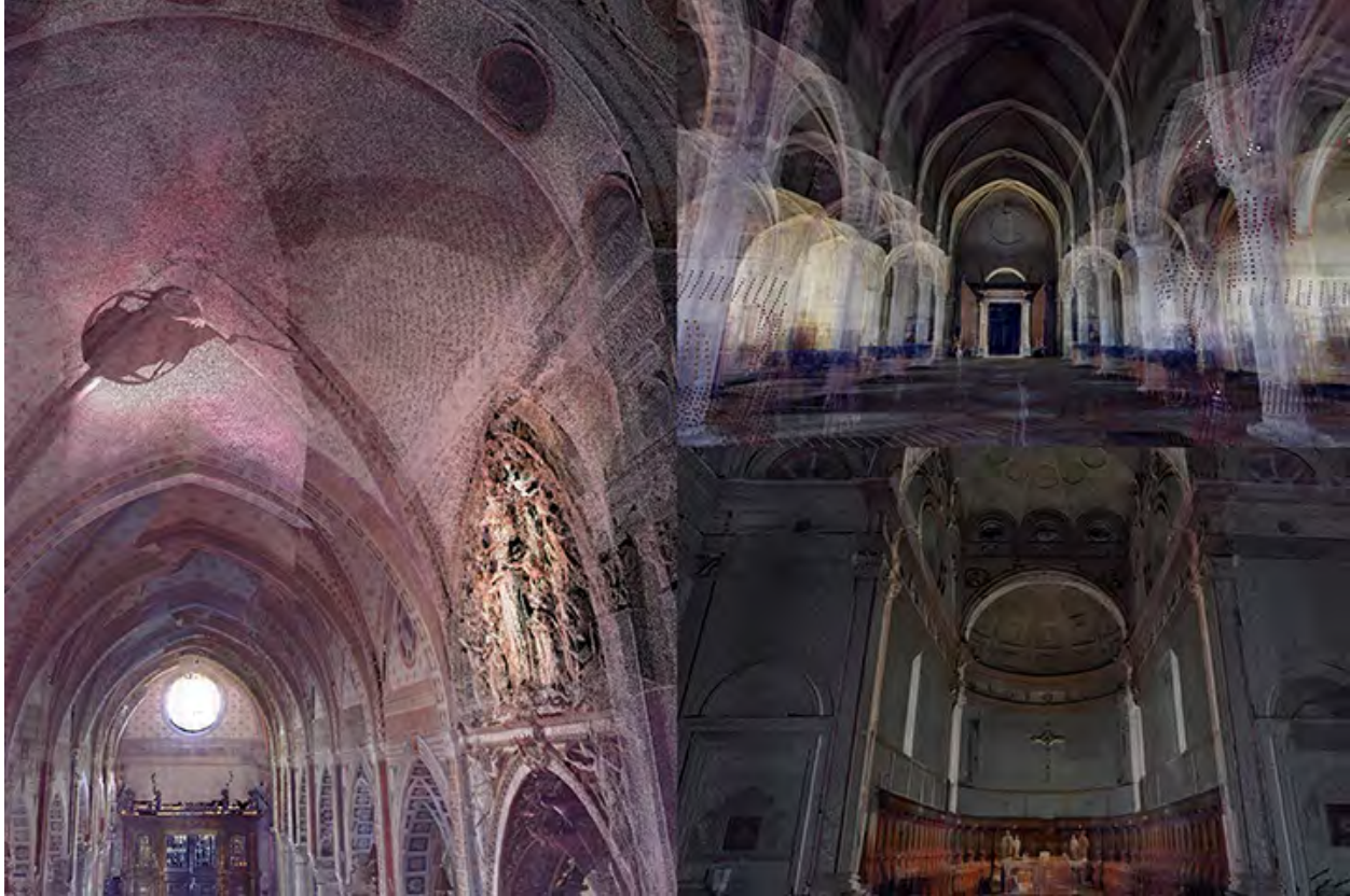
Figure 6. Different internal views of Immersive point cloud visualization in 8K of the Basilica Santa Maria Delle Grazie VR application. © F.Fischnaller.
