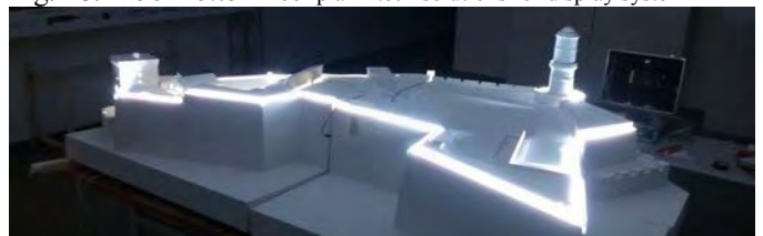
Fig. 19. 3D printed model A: 210x190x30/54 cm, with special led lighting system integrated inside the model. Photo: UNIRC
